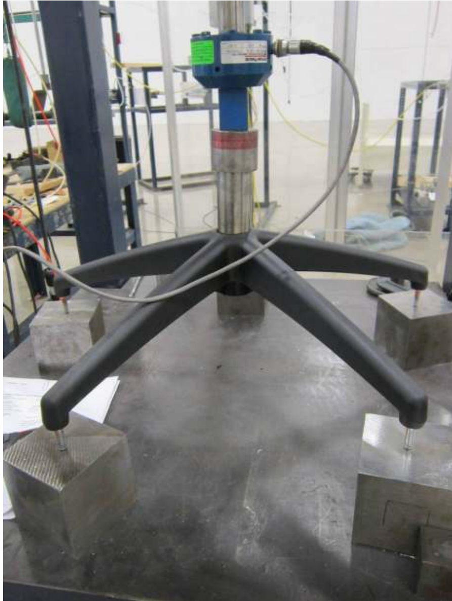
Base Test – Static
