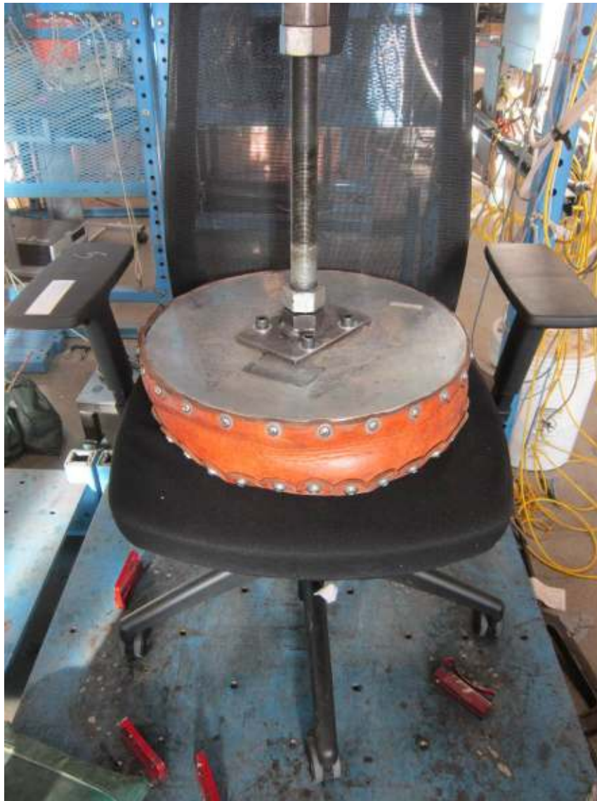
Seating Impact Test
