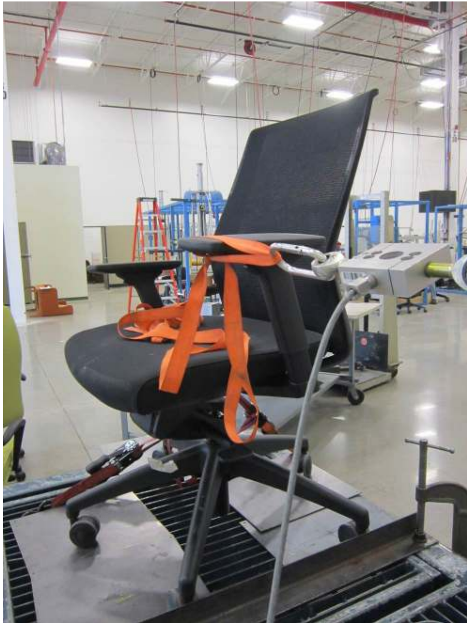
Arm Strength Test- Horizontal-Static
