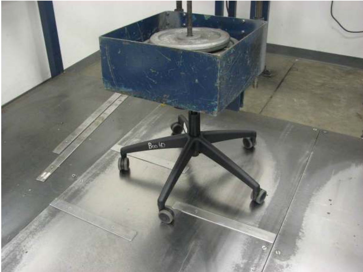
Caster/Chair Base Durability Test - Cyclic
