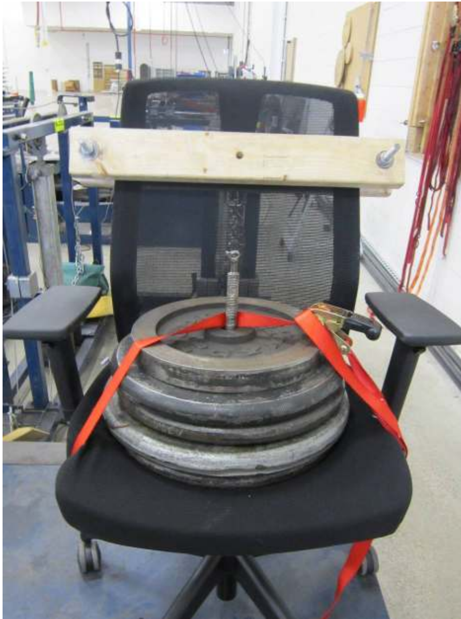
Tilt Mechanism Test-Cyclic
