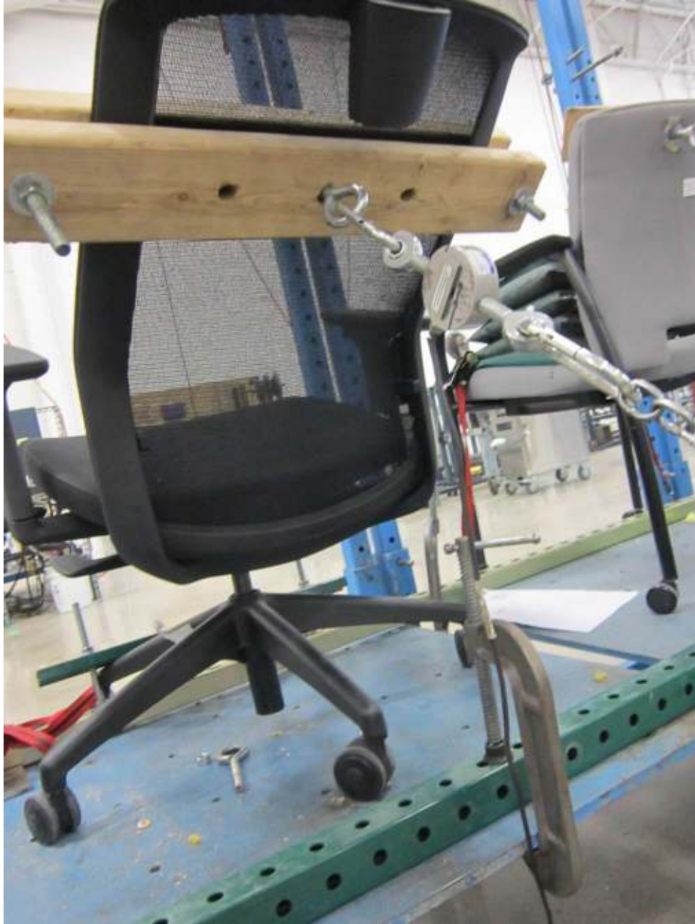
Back Strength Test
