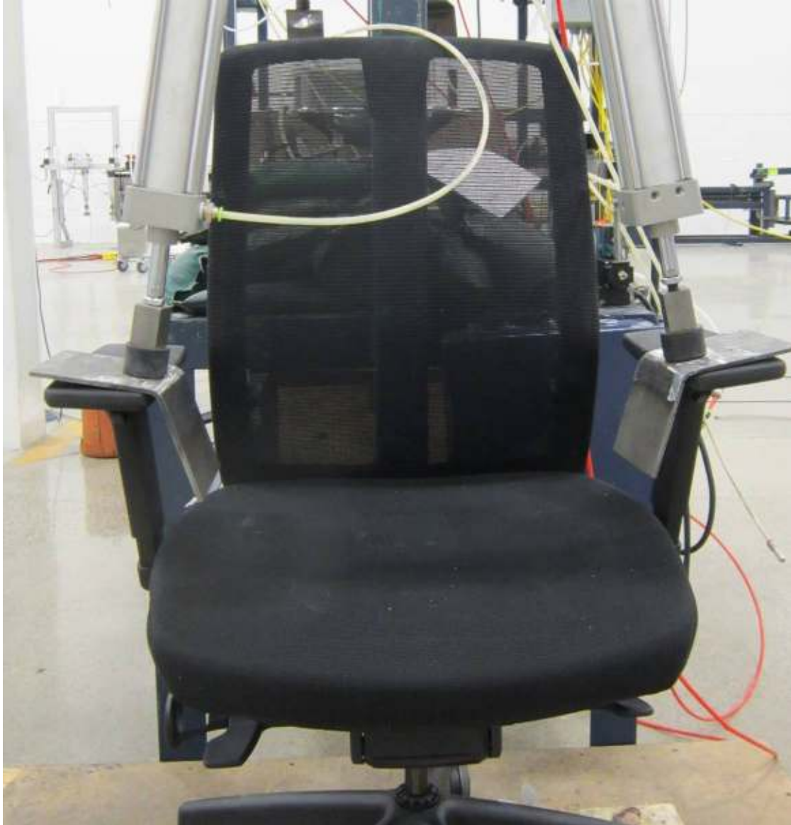
Arm Durability Test – Cyclic
