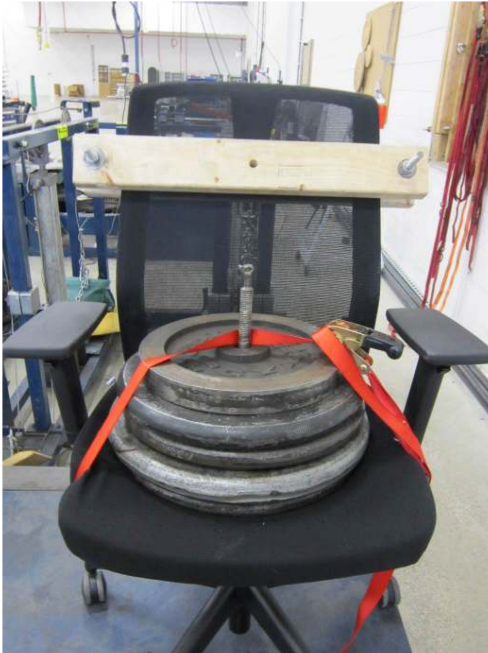
Back Durability Test-Cyclic
