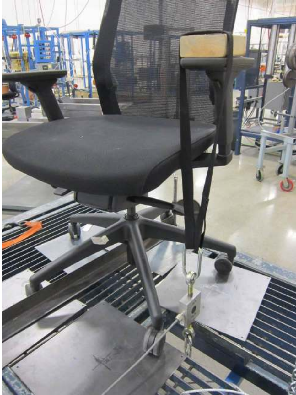
Arm Strength Test Vertical-Static
